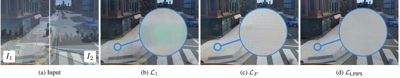
Figure 5: Training with \ell_1 distance led to low-frequency artifacts (b), and using squared distance between VGG features led to checkerboard artifacts (c). We hence train our synthesis model using LPIPS, which produces good results (d).
