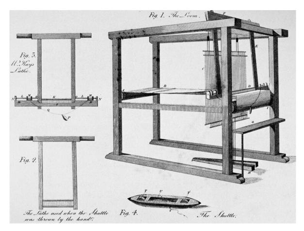
John Kay's 1733 Patent for the "New Engine or machine for Opening and Dressing Wool". This patent introduced the "flying shuttle" to the loom. The introduction of the shuttle allowed looms to be operated by a single laborer, and made loom production fast and efficient enough to facilitate its role in the industrial revolution. https://www.britannica.com/biography/John-Kay (https://www.britannica.com/biography/John-Kay)
