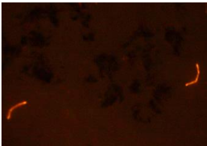
Figure 2: Example of Nile Red fluorescence from the Fall Creek 3 sample.
