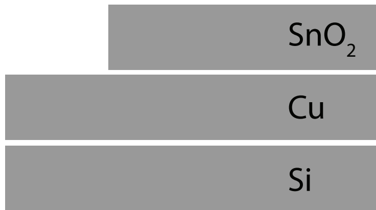
Fig. 3. Cu is deposited on \text{SiO}_2/\text{Si} . With some areas masked and others unmasked, \text{SnO}_x is deposited on top of the Cu layer.
