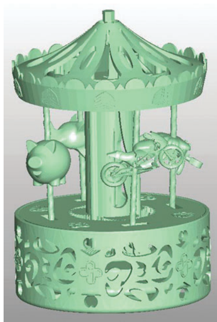
Figure 6. A rotational carousel with a flywheel at the bottom driven by a shaft located at the top. A planetary system steps up the energy input to the flywheel. A bevel gear system is attached to a support column and drives the reciprocating motion of the individual figures. The bevel system is mounted to an epicyclical gear set to reduce the rotational speed of the figures. 2
