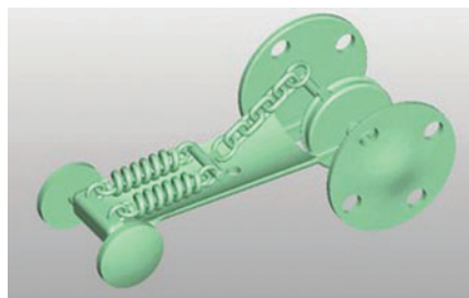
Figure 5. A pull toy spring car. The back axle is connected with a chain to two springs, which extend and drive the rear wheels for locomotion. 2
