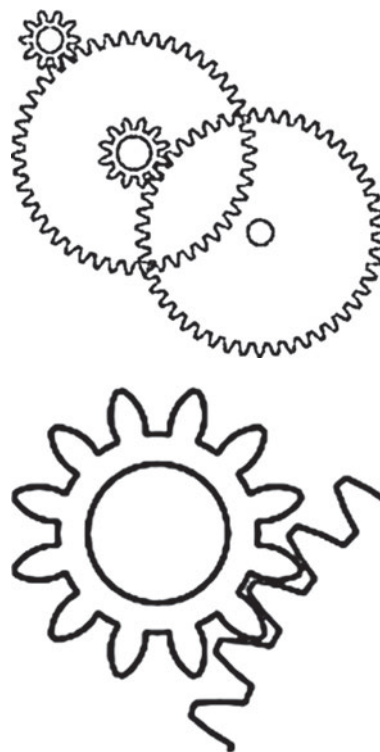
Figure 2. Gearing system of push toy car. Design rules can result in parts of gear mesh being slightly welded together and must break free during initial use.
