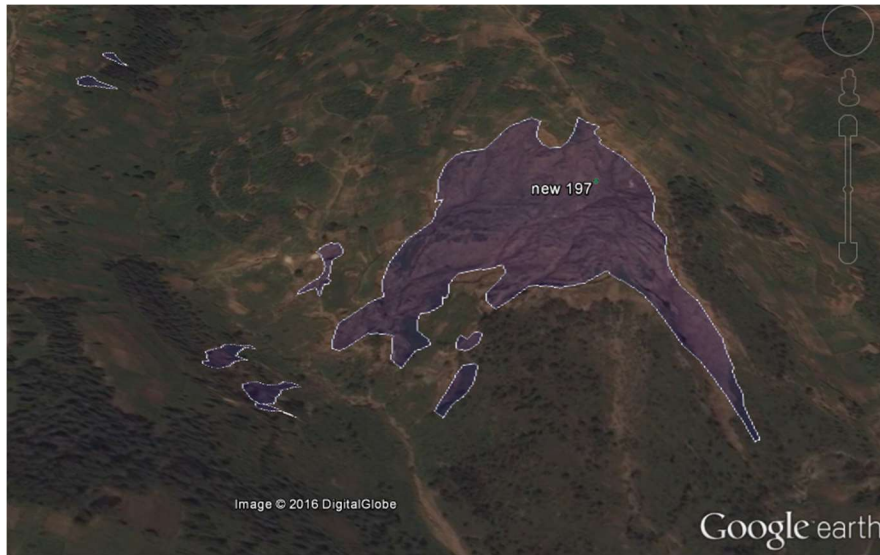
Figure 7. Example of polygons marking landslides in Google Earth. Each area identified as a landslide scar is outlined with a polygon to approximate the shape and area covered by the slide. Largest landslide is about 181 meters across, and 170 meters top to bottom
