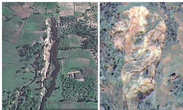
Figure 6. Examples of two recent landslides in the study area shown in WorldView/Google Earth satellite imagery. The color of the bare earth and the texture of the landslide scar stands out in contrast to the surrounding farmland or other ground cover.
