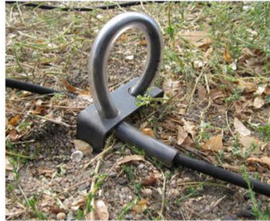
1d. Vinyl Tubing + Metal Bracket- used to secure MC 5' Loop and MC 2' Loop
