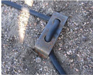
1c. Metal Bracket- used to secure the Eco-Counter's tubes
