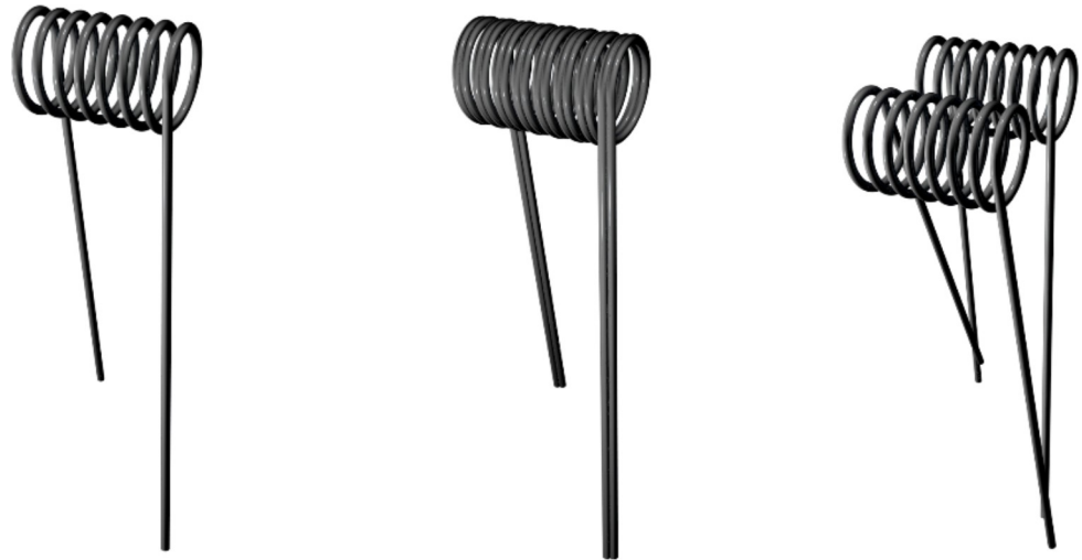
Fig 2. Illustration of single (left), parallel (middle) and dual coils (right). The parallel and dual coil contains two identical wires; however, the dual coils are wrapped individually with respective wicks. Each style can be oriented vertically or horizontally.
