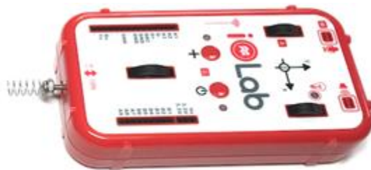
Figure 1. The IOLab, an inexpensive data acquisition device in a cart that can roll on its three wheels.
