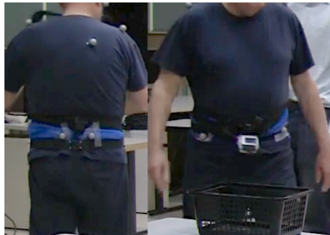
Figure 1. Inertial sensor, markers placement (back) and video camera attachment (front).
