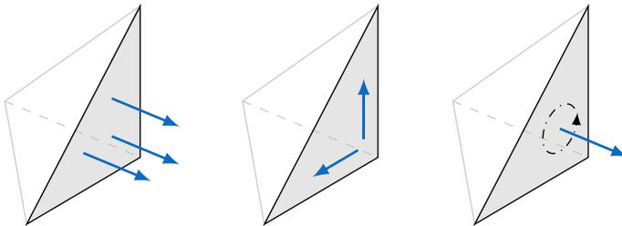
**Fig. 2** Classification of facet  $\text{dof}s$  in our new methods into three types: (1) normal velocity components in the form of  $\mathcal{BDM}^1$  facet  $\text{dof}s$ , (2) tangential facet velocities, (3) normal vorticity as  $\mathcal{RT}^0$  facet  $\text{dof}$
