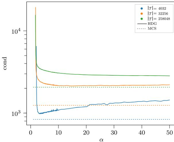
**Fig. 3** Approximate condition numbers of the corresponding  $A$  blocks of the HDG (solid lines) and the MCS (dotted lines in the same color) method on different meshes. Different values of  $\alpha$  on the  $x$  axis and approximate condition number (cond) on the  $y$  axis
