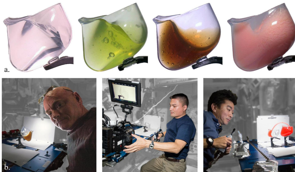
Fig. 2 The Capillary Beverage experiment “science”. a Space cup with various beverages: bubble-free water, limeade, Kona Black coffee with small bubbles and undissolved coffee particles, and peach-mango smoothie. b NASA astronauts S. Kelly, K. Lindgren, and JAXA astronaut K. Yui on ISS.
