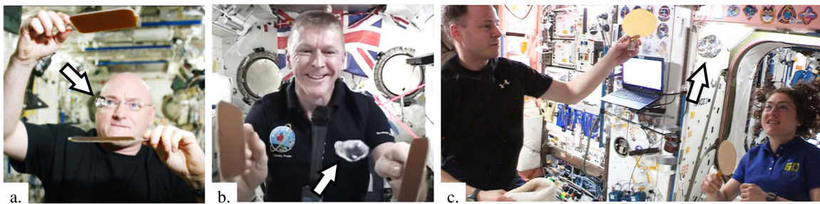
Fig. 11 Demonstrations of super-hydrophobic surfaces by ISS crew. ISS astronauts a S. Kelly 58 , b T. Peake 59 , and c N. Hague and C. Koch 28 demonstrate large length scale non-wetting phenomena with super-hydrophobic paddles and water blobs of ~ 10, 30, and 250 mL, respectively (see white arrows).
