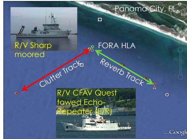
**Figure 1: Map showing placement of the Five-Octave Research Array (FORA) horizontal line array (HLA) during the 2013 TREX data collection. The R/V Sharp collected monostatic sonar data from the HLA while R/V CFAV Quest towed an echo repeater (E/R) along the clutter and reverb tracks.**
