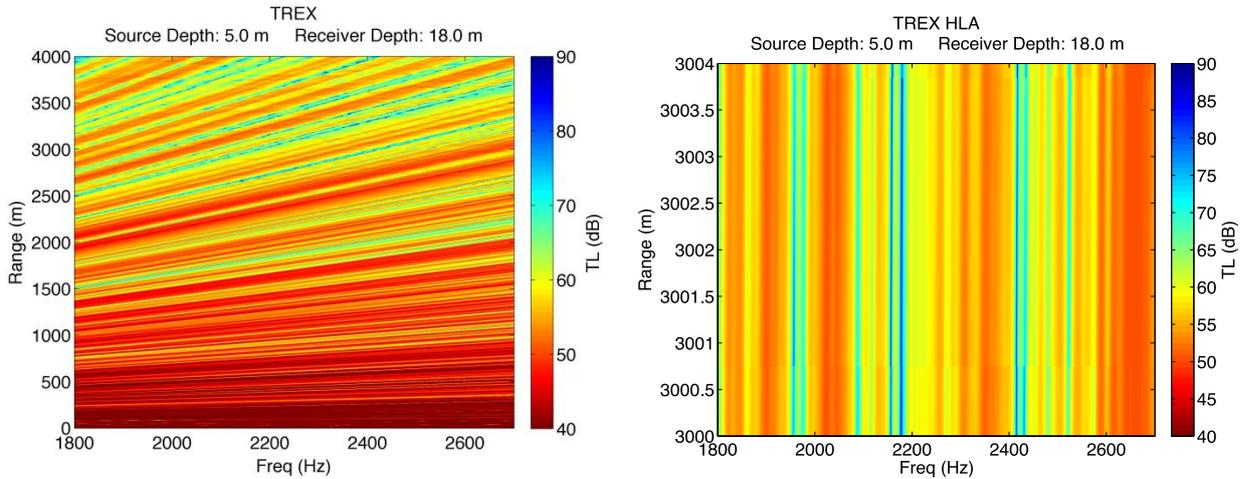
**Figure 3: Ray propagation simulation for HLA with spacing equivalent to the TREX array. Left-hand side : range-frequency striations for 4000 meter separation. Right-hand side: Range extent of actual array (~ 4 meters) in which striations appear vertical.**
