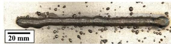
Fig. 4 Bead appearance in GMA-WAAM of Ti-6Al-4V alloy
