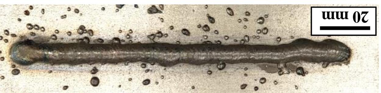
Fig. 4 Bead appearance in GMA-WAAM of Ti-6Al-4V alloy
