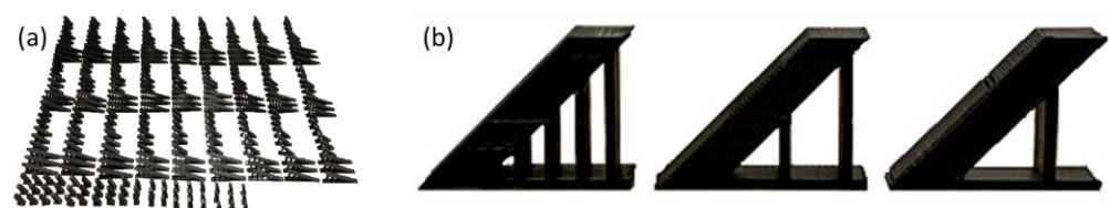
Figure 4. Printed 3D objects of (a) all objects and (b) with 45° inclination angle and support spaces of 5 mm, 10 mm, and 15 mm.
