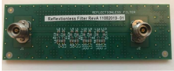
Figure 7. PCB implementation of reflectionless LPF with four cascaded sections and equivalent filter order n=12 with corner frequency 188 MHz.
