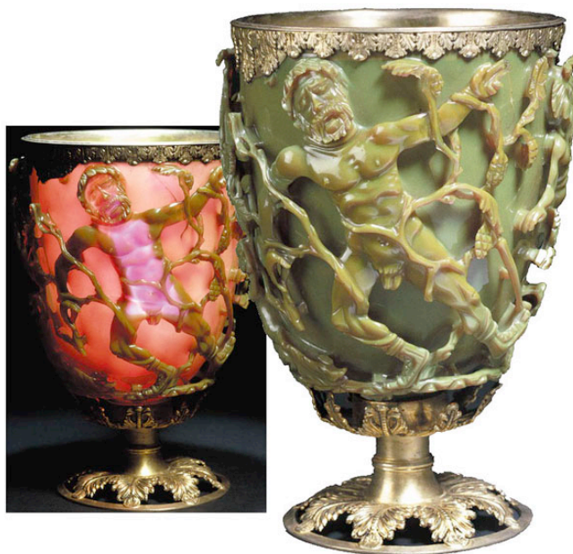
Figure 1.1 – The Lycurgus Cup showing the dichroic nature of the glass. The 300 ppm silver nanoparticles reflect an opaque green (seen right) while the 50 ppm gold nanoparticles give a translucent red color when light is shined through the glass (seen left). 4,74
