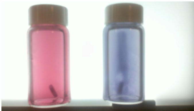
Figure 3.11 – Picture of vials containing \text{PC}_{30} growth (left) and \text{PC}_{95} growth (right). Note the precipitate in the \text{PC}_{95} sample
