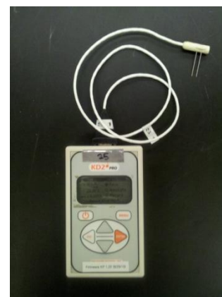
Photo 3: KD2 Pro thermal properties analyzer.
