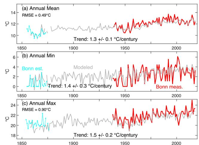
**FIGURE 6** Annual mean, minimum, and maximum water temperature trends based on measurements (red: Bonneville; cyan: Bonneville estimated from Astoria) and the composite model (gray: Vancouver). A linear trend (based on model results) is included for each metric with the standard error of the slope of the regression. RMSE, root mean square error. [Color figure can be viewed at [wileyonlinelibrary.com](http://wileyonlinelibrary.com)]
