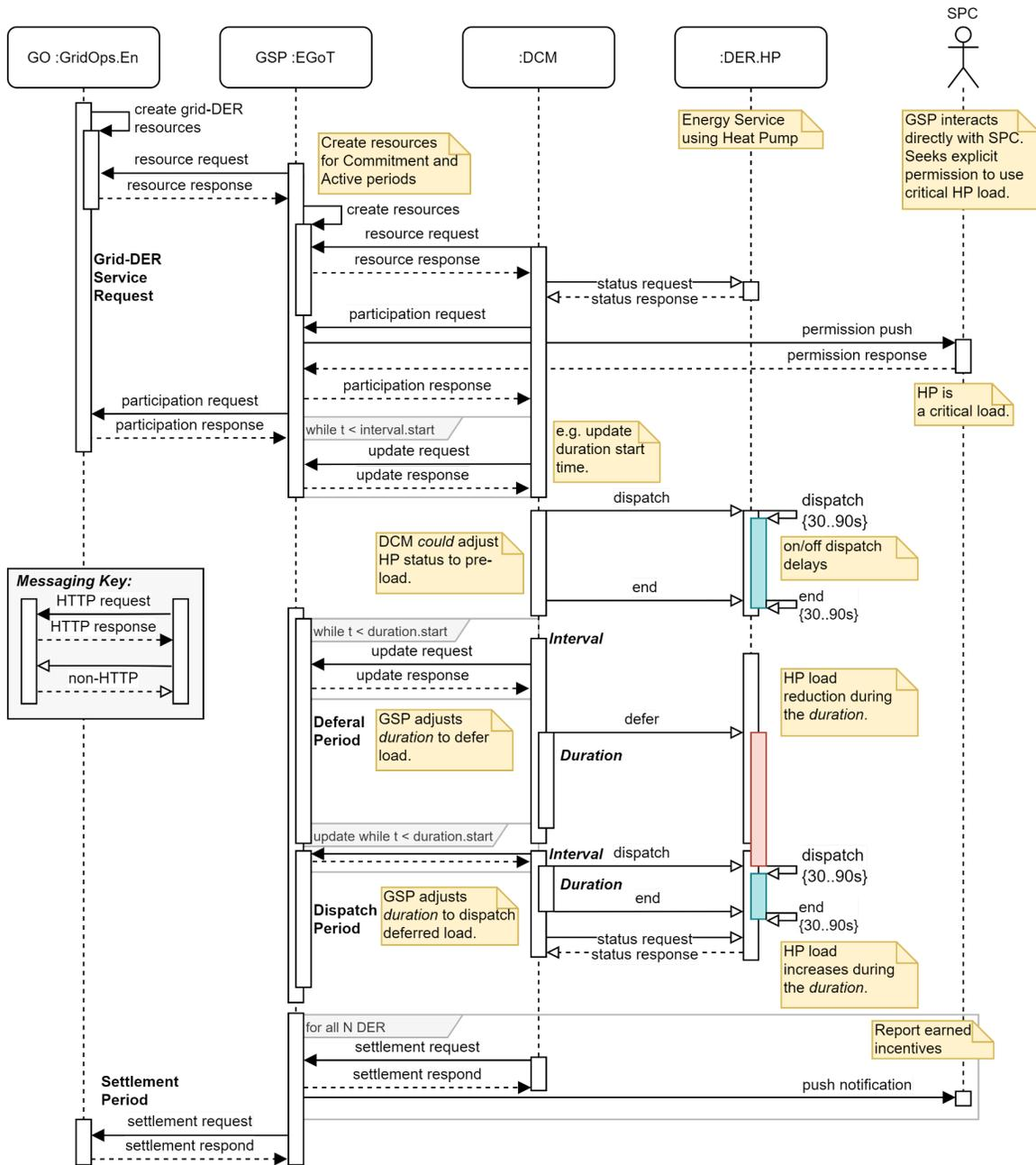
**Figure B.3** Sequence diagram for grid-DER Energy Service provided by a Heat Pump (HP) HVAC system. HP operation is deferred from one period to a later period. In anticipation of deferral, the DCM operates the HP at an adjusted setpoint (e.g. lowered if in cooling mode).
