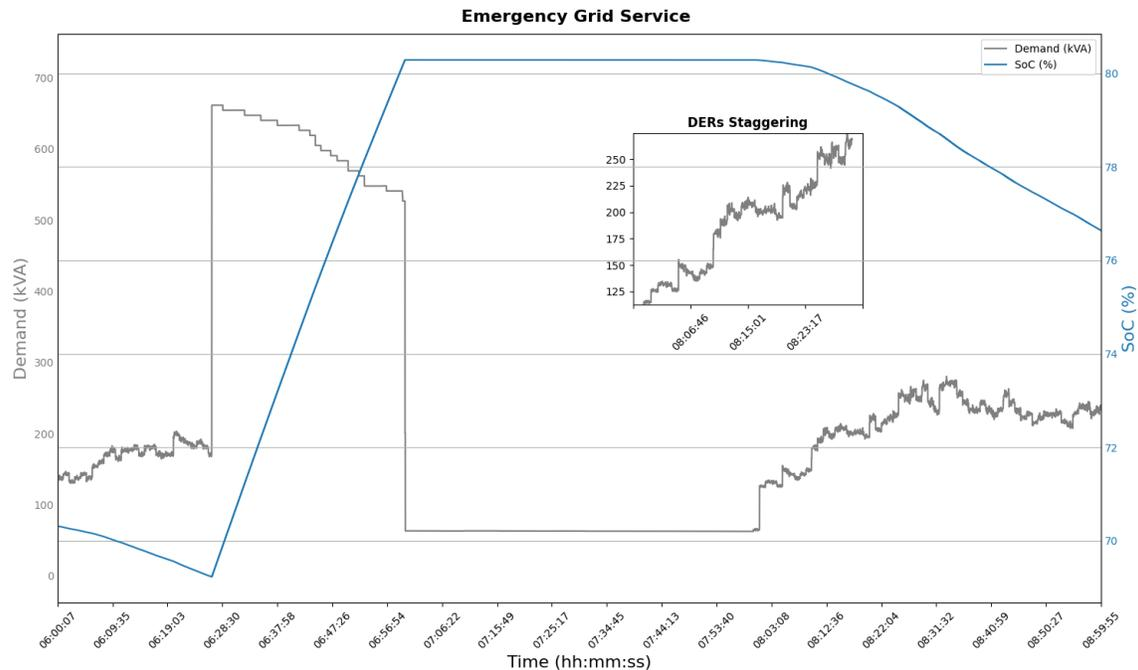
**Figure C.1** Demand (kVA) and State of Charge (SoC) of the Aggregated DERs in a Blackstart grid-DER service Scenario. The main blackstart service characteristics are shown: energize, defer, and return to normal operation in a staggering manner.
