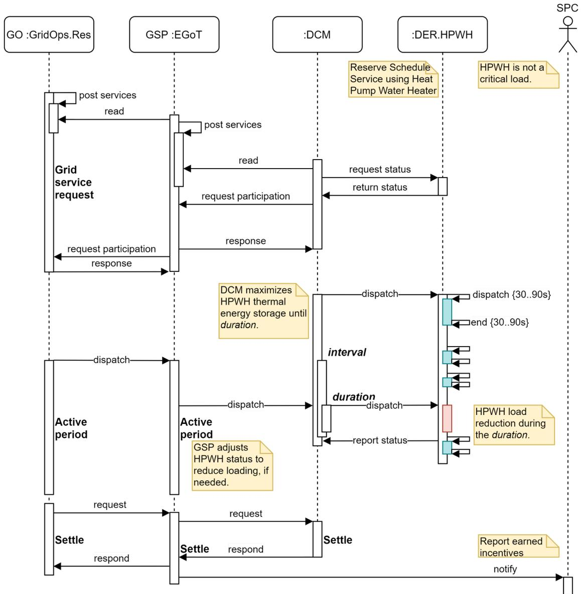
**Figure B.5** Sequence diagram for grid-DER Reserve Service provided by a heat pump water heater (HPWH).
