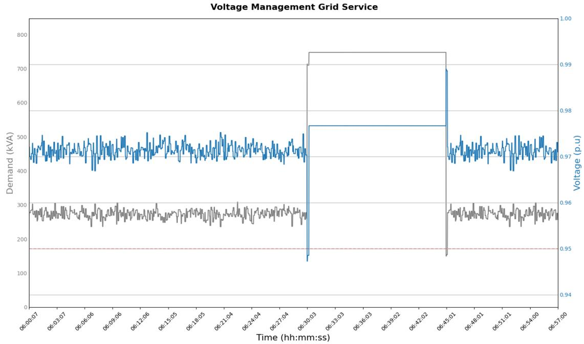
**Figure C.4** The demand in kVA and voltage (p.u) of the aggregated BIS DERs. The response to the voltage drop below 0.95 is > 3 seconds due to GridAPPS-D; it retrieves measurements every three seconds.
