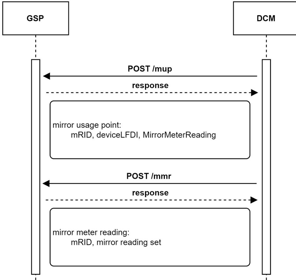
**Figure 5.6** DCM mirror meter reading set for *Flow Reservation* response validation.
