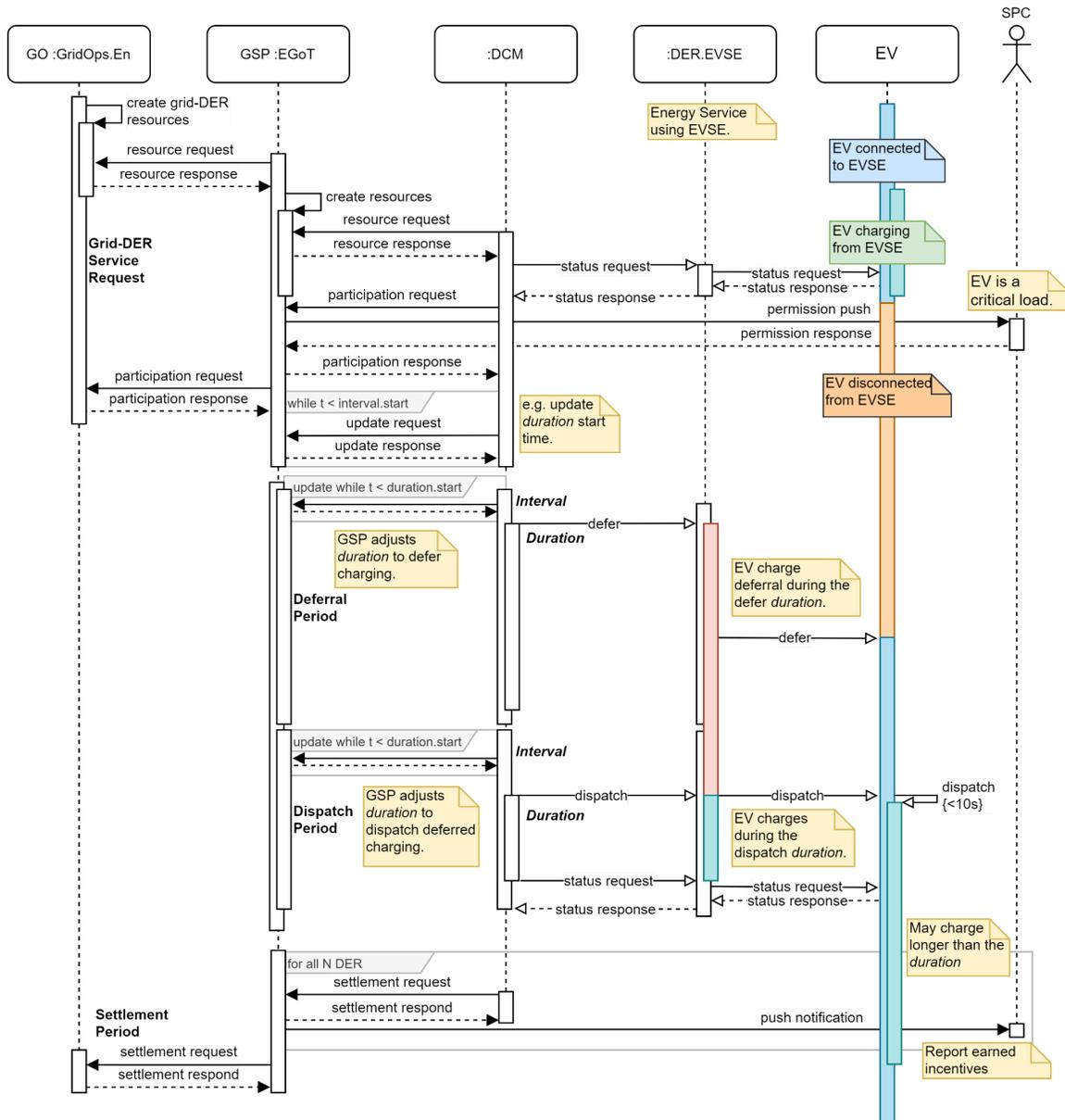
**Figure B.4** Sequence diagram for grid-DER Energy service provided by electric vehicle service equipment (EVSE). Charging requires the EV to be plugged into the EVSE. Operation is deferred from one period to a later period.
