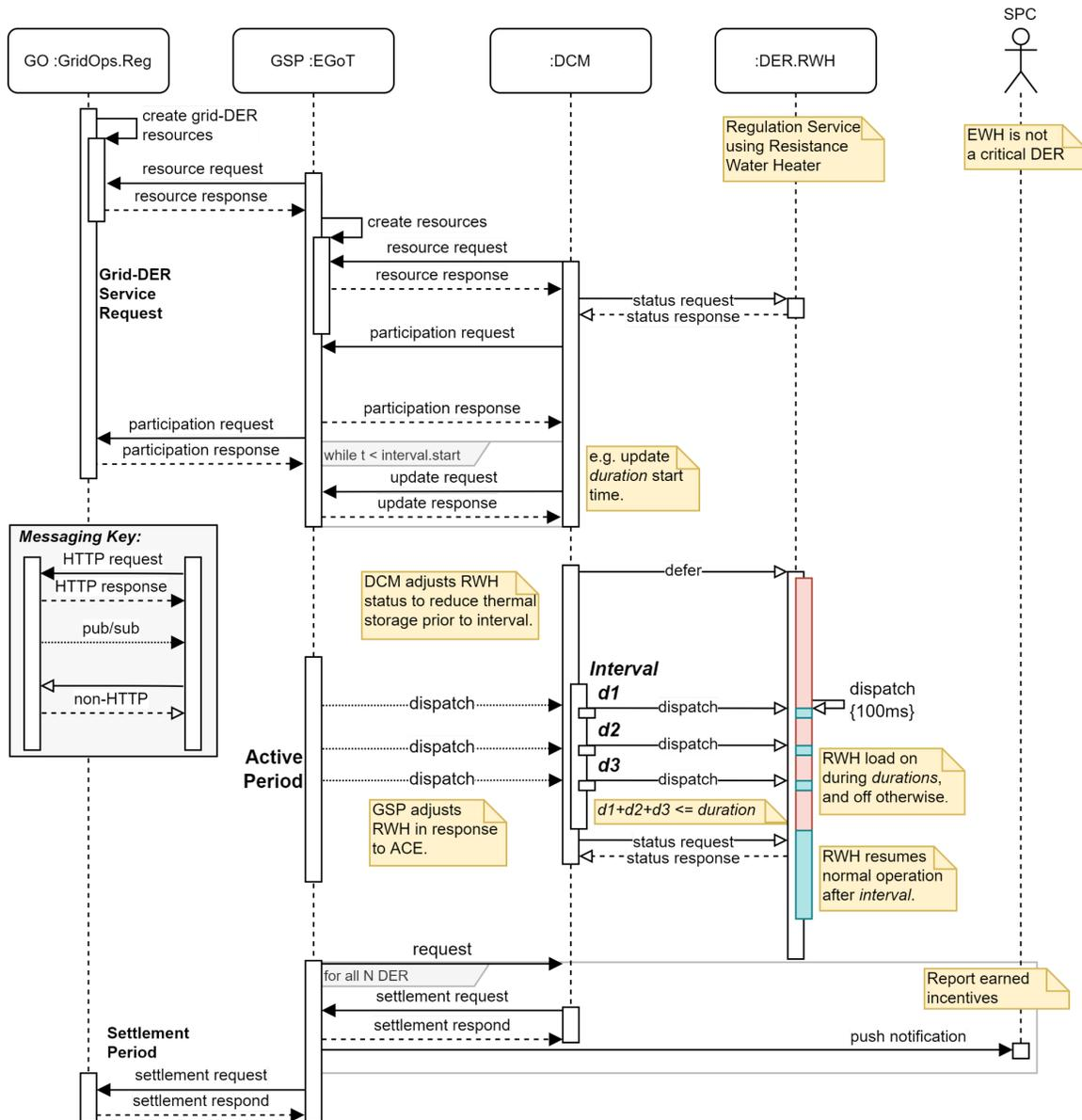
**Figure B.6** Sequence diagram for grid-DER Regulation service provided by an electric resistance water heater (EWH). The DCM reduces EWH loading prior to the regulation period. Since the EWH is interruptible, the GSP may dispatch the EWH as needed in response to positive ACE deviations.
