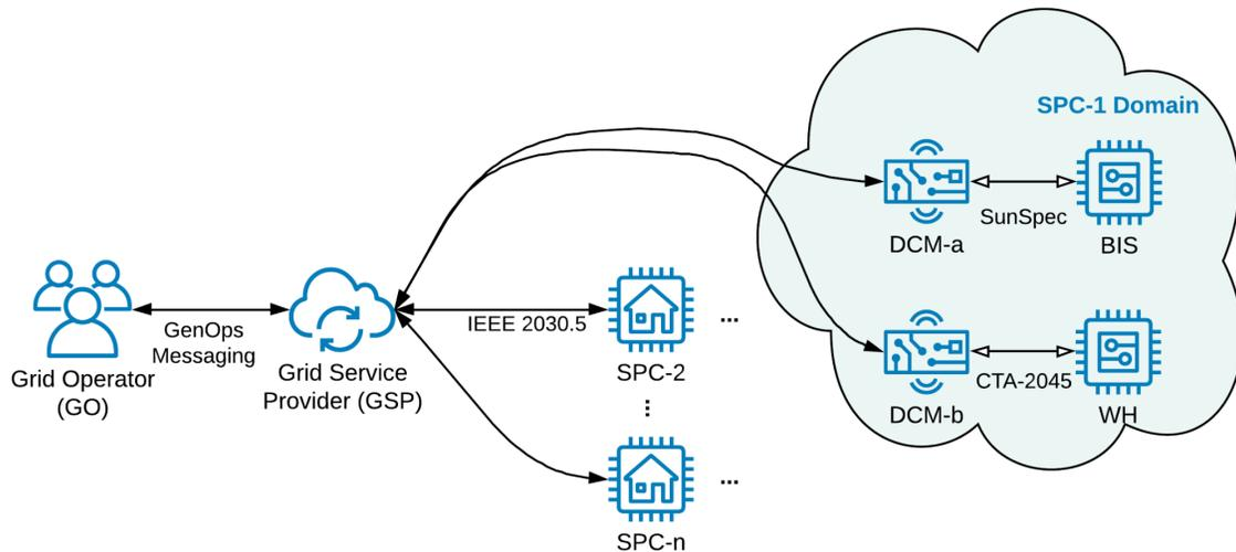
**Figure 3.1** The communication paths between system actors using different protocols. This IP focuses on the GSP-DCM pathway, which uses a subset of IEEE 2030.5 smart
