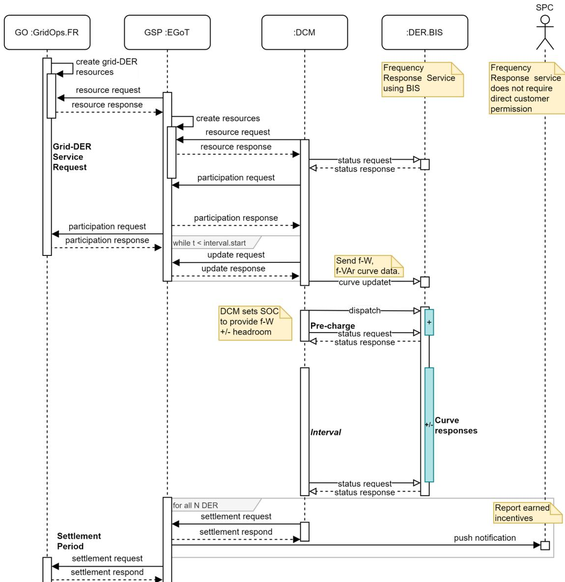
**Figure B.10** Sequence diagram for Frequency Response grid-DER service provided by a battery-inverter system (BIS). The service is provided by automatic response according to f-W and f-VAr curves loaded into the BIS.
