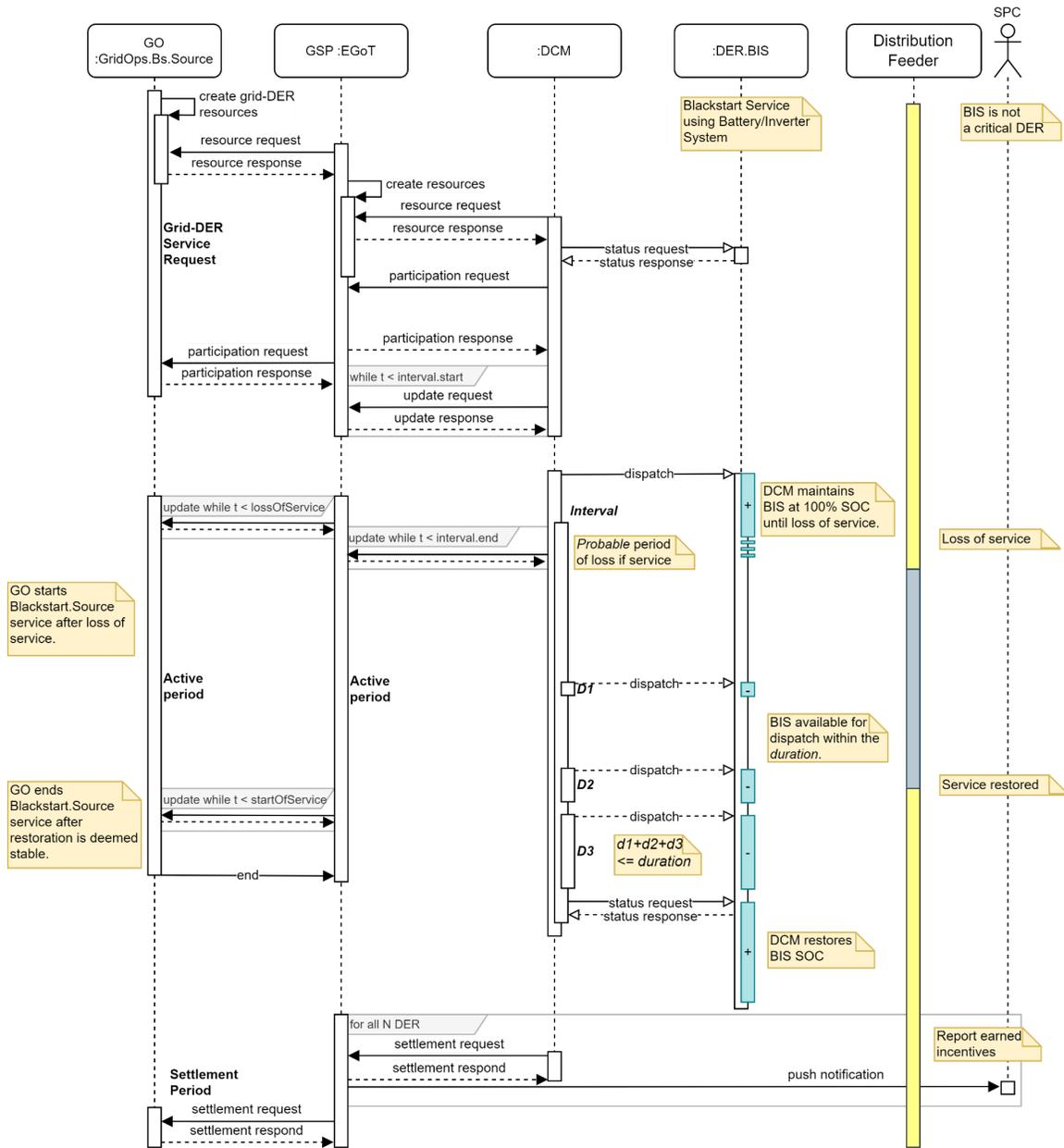
**Figure B.8** Sequence diagram for Grid-DER Blackstart Service provided by a battery inverter system (BIS). The DCM maintains the BIS state of charge (SOC) until loss of electrical service. The BIS may then be used by the GO to help support restoration.
