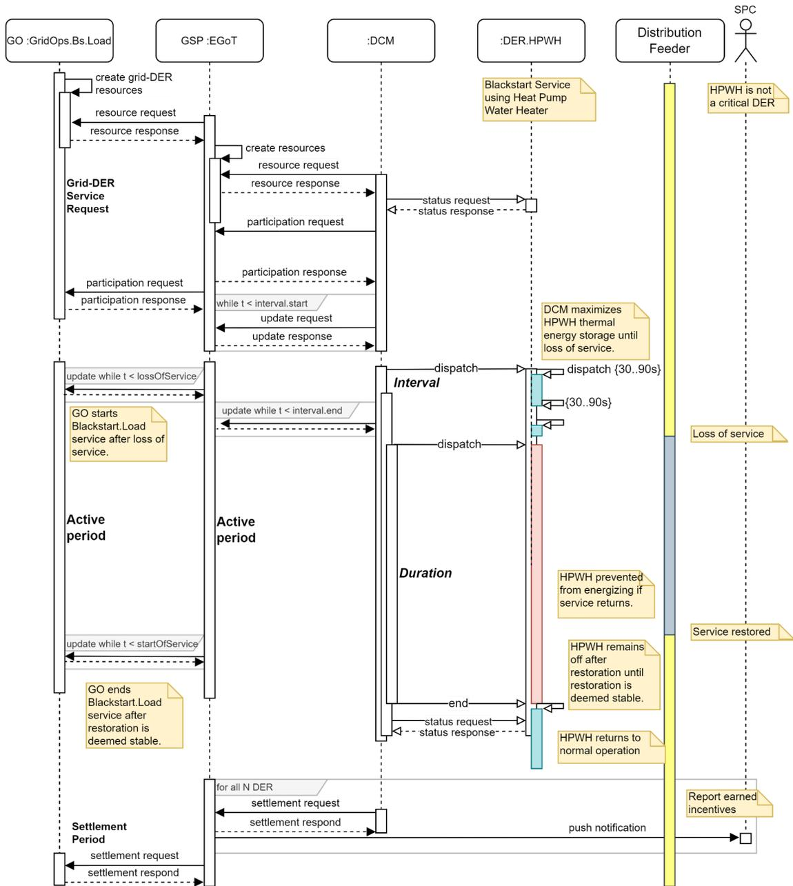
**Figure B.7** Sequence diagram for Grid-DER Blackstart Service provided by a heat pump water heater (HPWH). The HPWH is a non-coincident, non-critical load that presents high in-rush at startup. Deferring the load until after electrical service restoration helps the GO re-energize the feeder.
