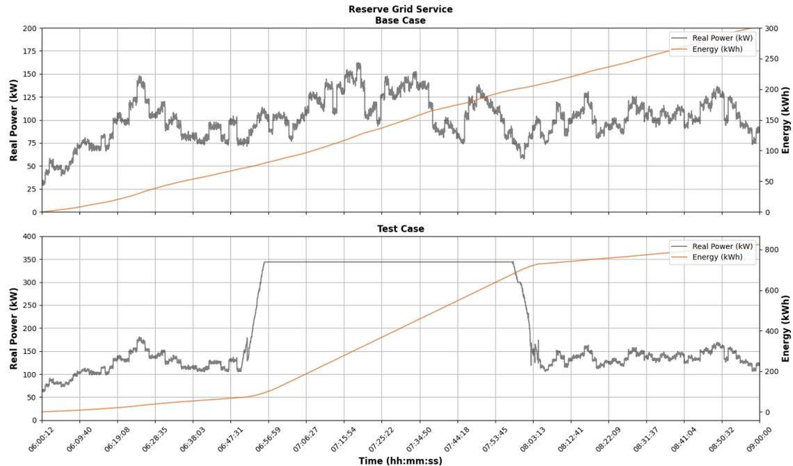
**Figure C.3** DERs demand (kVA) and Energy consumption (kWh) during a reserve grid-DER service. The top plot represents the base case where no grid-DER service is simulated. The lower plot represents the test case wherein DERs simulate an augmentation of generation capacity.
