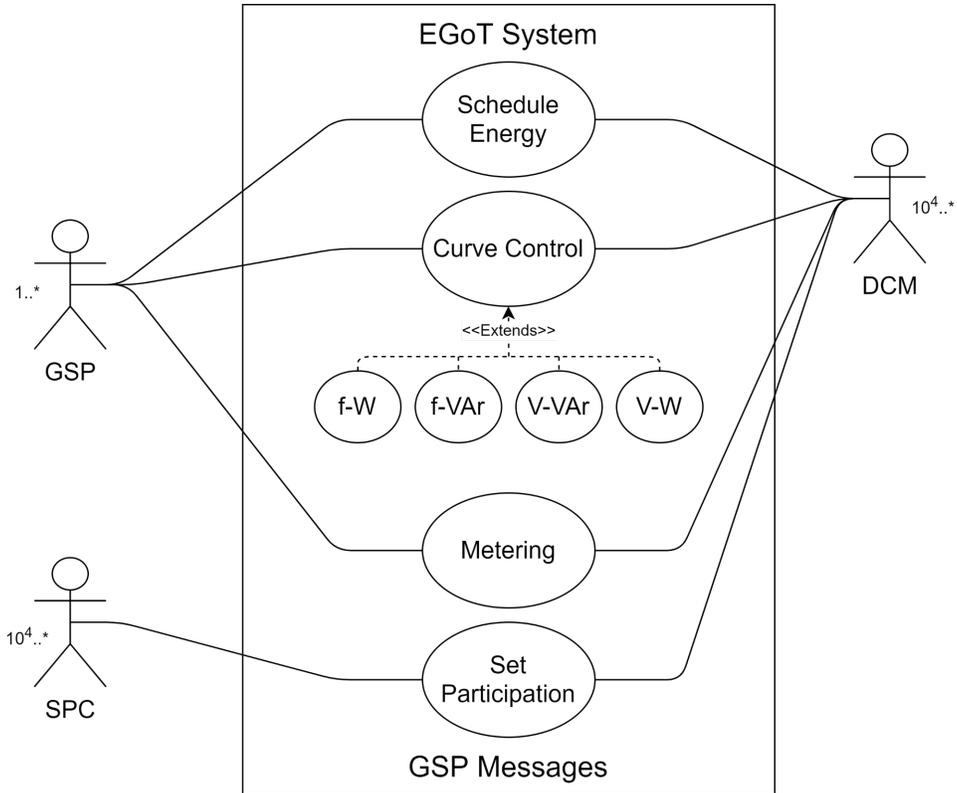
**Figure B.2** Use Case diagram for the EGoT DERMS, which manages information exchange between a GSP and one or more and large numbers of DERs. DCM agents act on behalf of SPCs to request IEEE 2030.5 resource services from a GSP. Tens to hundreds of thousands of DERs will need to be aggregated to provide grid-DER services that have meaningful impacts on power systems operation.
