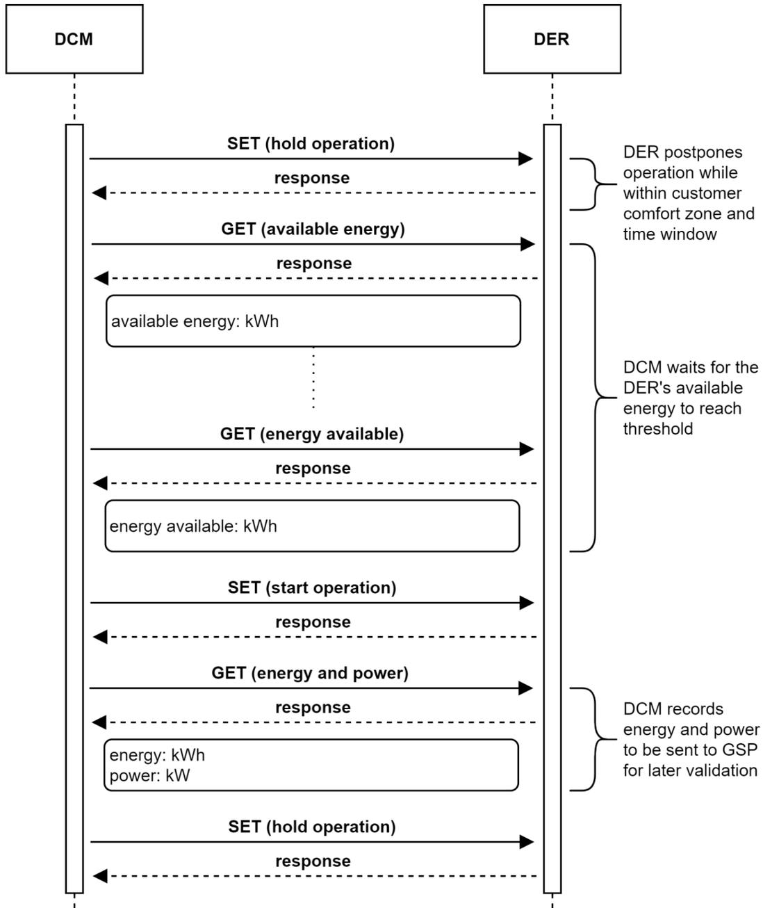
**Figure 5.7** DCM *Flow Reservation* implementation process; gateway service to the DER.
