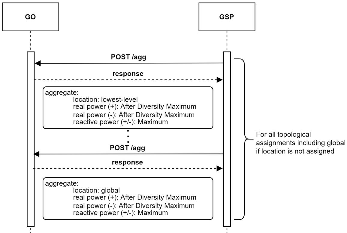
**Figure 5.1** Simplified GSP characteristics for GO registration. The above sequence diagram is generic; this IP does not specify IEEE 2030.5, or any other protocol, for GO-GSP information exchange.
