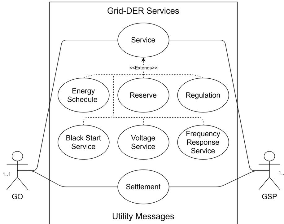
**Figure B.1** Use case diagram for grid-DER services showing message exchange between the GO and the GSP.
