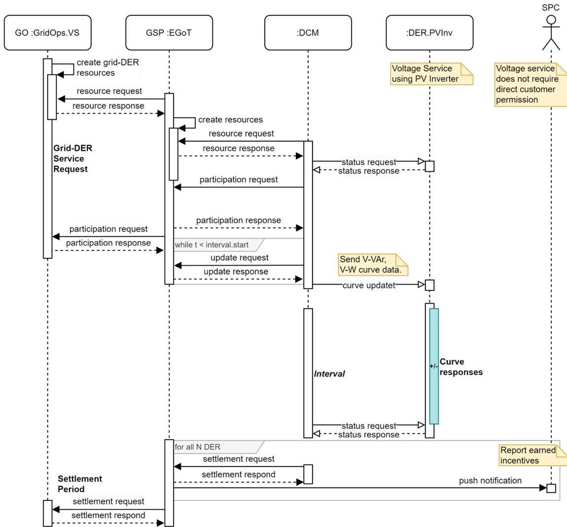
**Figure B.9** Sequence diagram for grid-DER Voltage Management Service provided by a Photovoltaic-inverter system (PVInv). Service is provided by automatic response according to V-VAr and V-W curves loaded into the PVInv. SPC permission for this service would be granted when the SPC initially registers with the GSP program. A PV system coupled with a battery would undergo some additional pre-charge steps, similar to those shown in Figure B.10.
