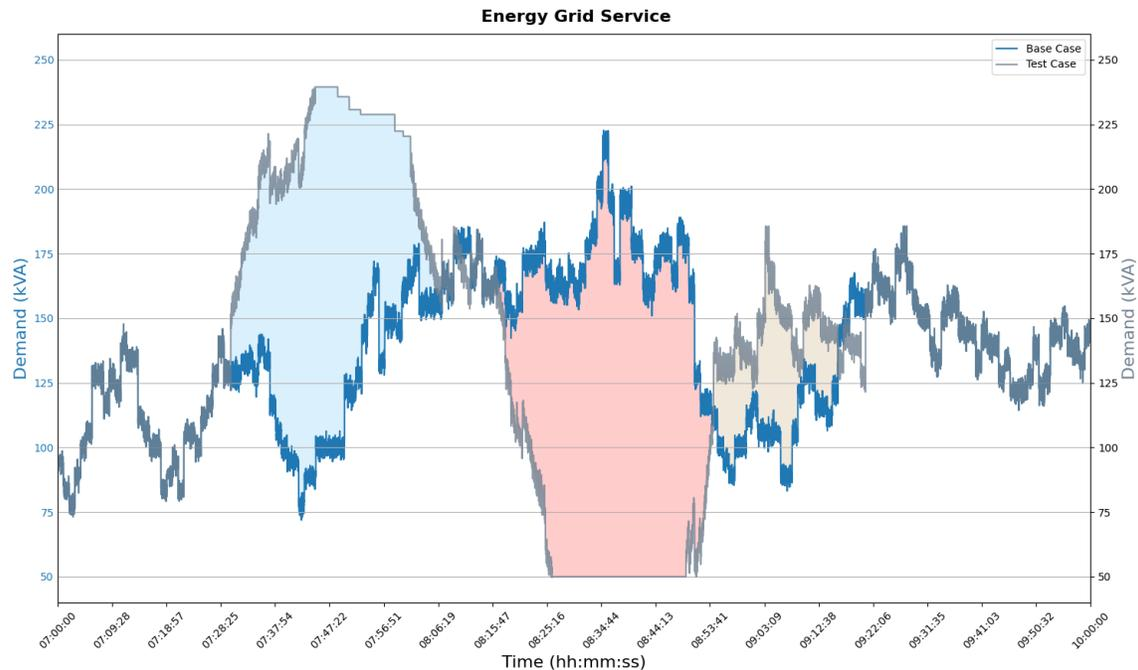
**Figure C.2** Behavior of DERs demand in kVA during Energy Service. The blue line represents the base case. The gray line represents the test case.
