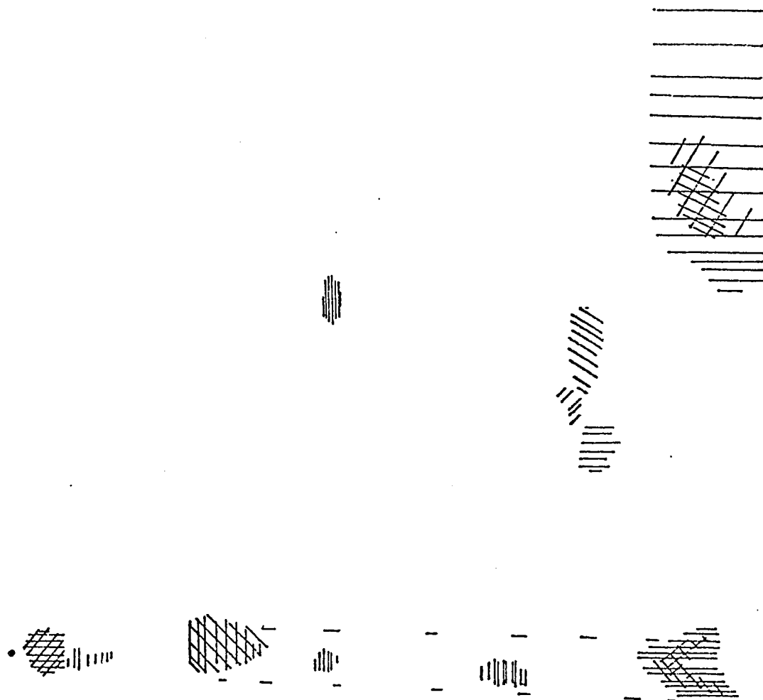
Fig. 8. Two-dimensional (TLC) chromatogram of concentrated Algal products from S. capricornutum , grown w/o Cu. The first separation is in the vertical direction with ethyl acetate, second separation, horizontal direction from left to right with n-butanol, formic acid and water 4:1:1 v/v/v. Symbols represent the following: ||| = ninhydrin positive reaction, ≡ = fluorescent activity, // = visible, \\\ = iodine staining.
