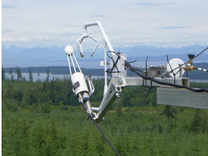
Figure 3 Eddy Covariance device used to measure carbon fluxes
