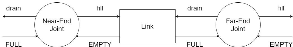
Fig. 9: A First-In-First-Out (FIFO) Buffer, Near-End Joint - Link - Far-End Joint.
