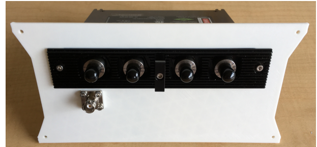
FIG. 14. Picture of the front panel, showing SPCM-AQ4C and gate signal BNC input affixed.
