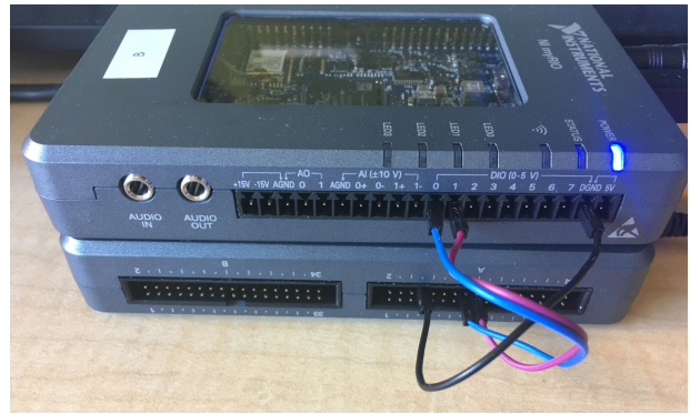
FIG. 29. Picture of the myRIO-to-myRIO configuration used to characterize the CCU performance. DIO lines from test signal generator are connected directly across to DIO lines for CCU FPGA. DGND lines are also connected.
