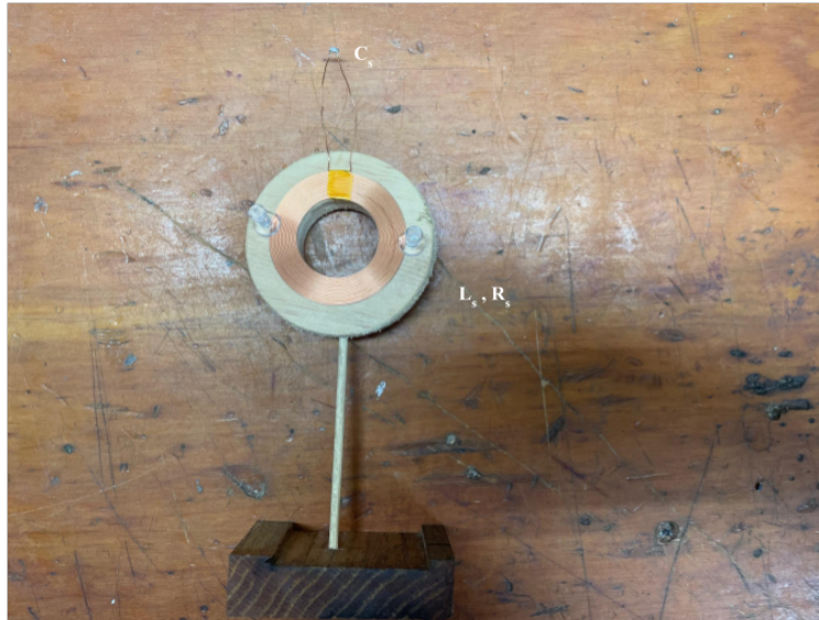
Fig. 7: The Experimental Air-Core Relay Setup. Note that parameters indicated were measured to be L_s = 50.9\mu H , R_s = 0.9\Omega , C_s = 15.5nF
