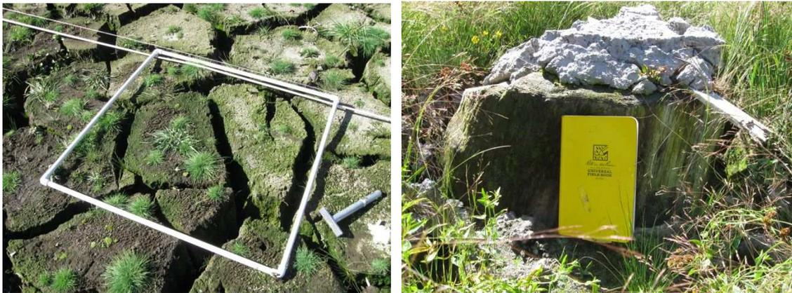
**Fig. 1.** Examples of the physical characteristics of ripening. Left (a): cracking as a result of dehydration of exposed sediment. Right (b): Subsidence indicated by the isolation of sediment from the reservoir surface in the center of the reservoir.
