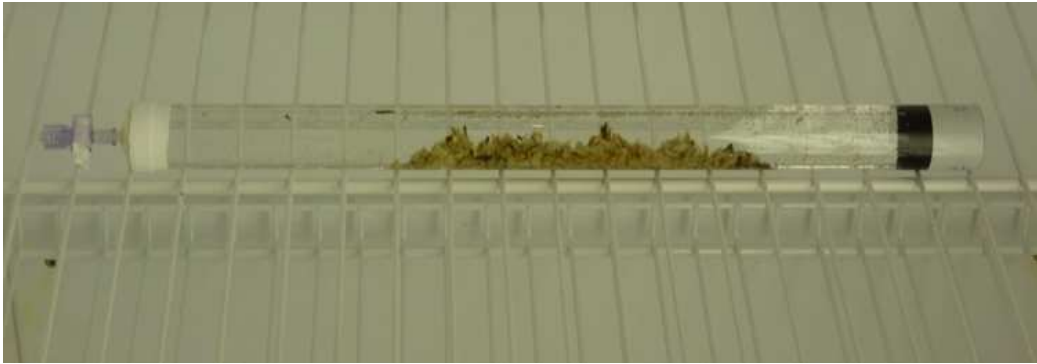
Figure 2.3: Quartz tube with periphyton and attached stopcock valve.
