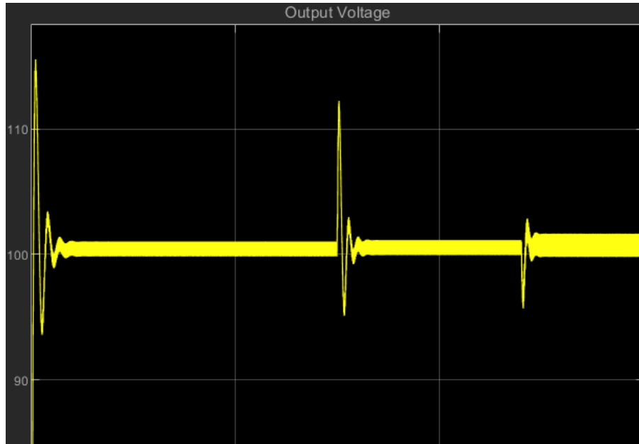
Figure 10: Boost converter closed loop output with input voltage and load disturbances
