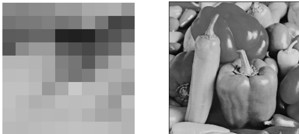
Figure 1.2. 10 \times 10 gray squares of varying intensity (left) and 256 \times 256 gray squares of varying intensity (right). The left image is a close-up of a small piece of the right image.
