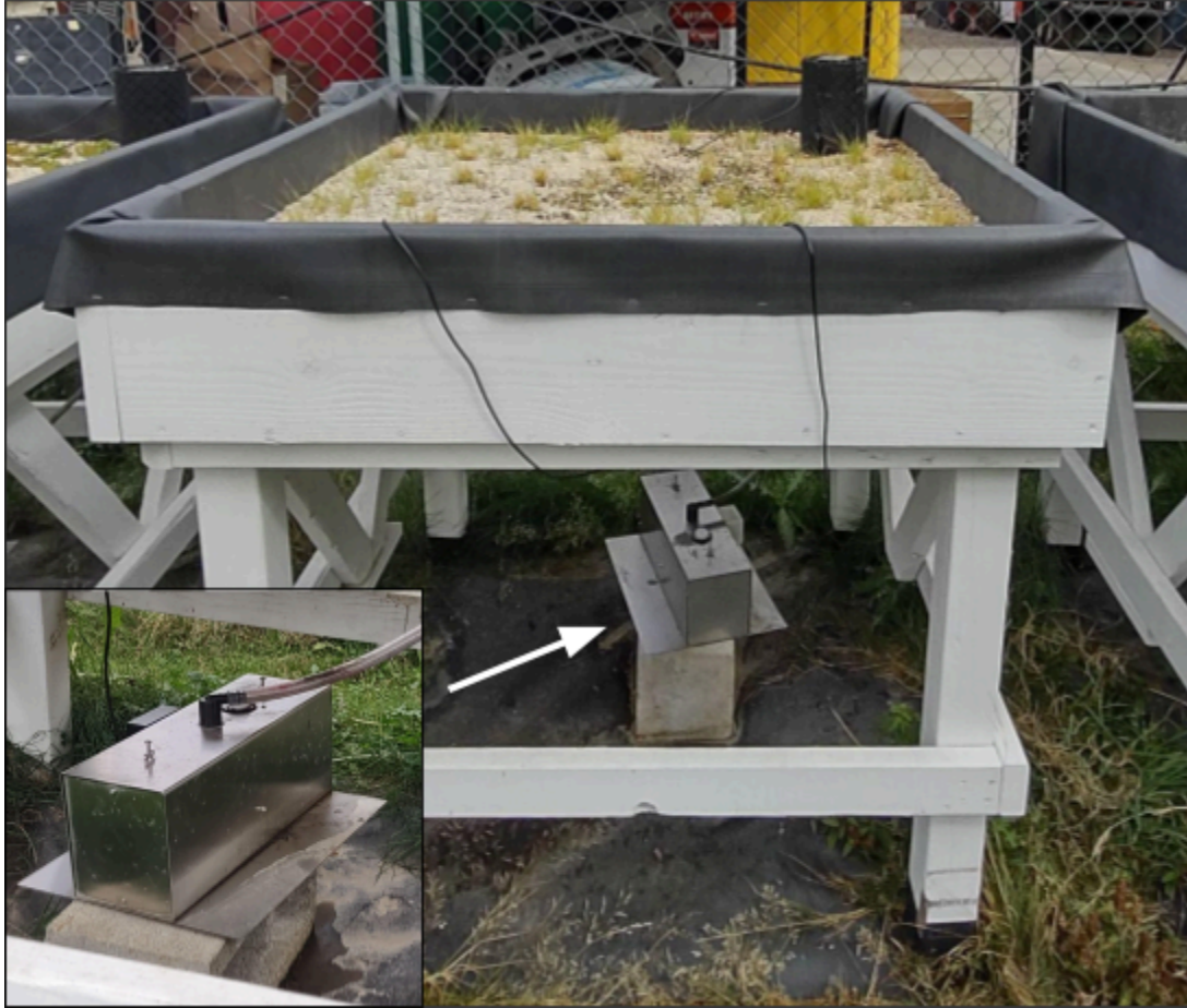
Figure 2. Photo of one out of seven trays and a closeup of the tipping bucket used to measure stormwater runoff (mL), located underneath each tray.
