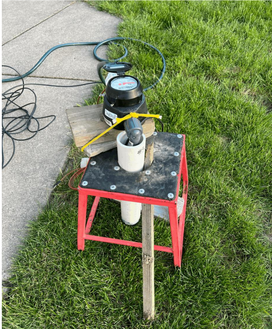
Figure 2: The image above shows my personal experience of calibrating the drain gauge device I constructed. As shown, a hose is attached to the Recordall badger meter which is recording the rate of water entering the drain gauge (GPM). The drain gauge is being held up by a variety of random objects creatively placed to keep the gauge upright. Not shown in this image is the CTD-10 sensor which is inside the drain gauge and the Zentra data logger giving me in time readings from the sensor.
