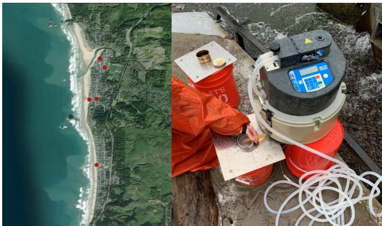
Figure 1. Left: Location of the five sample location sites in Cannon Beach, Oregon. Right: Sample collection set-up using an ISCO 6712 autosampler, orange five gallon buckets, sieves, custom sieve holders, and orange ponchos for sample collectors.
