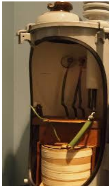
Fig. 2: Cutaway section of distribution transformer [4]
