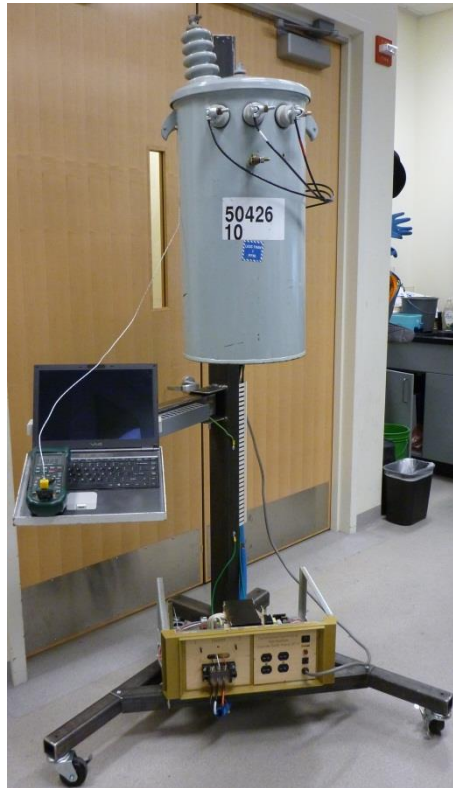
Fig. 15: Primary wiring of Transformer Monitoring Test Station
