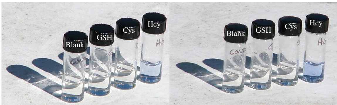
Figure 3.1 Response of MV^{2+} towards various thiols upon exposure to direct sunlight. Solutions of MV^{2+} (50 mM) were mixed with thiols (20 \mu M) in 0.5 M Tris buffer at pH 7, saturated with argon and exposed to sunlight. Pictures were taken at 1 min (left) and 2 min (right) after exposure to sunlight.
