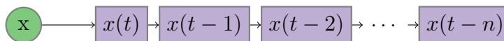
Figure 3.1: Diagram of an example delay line. The circle, x , is the input value and box x(t) represents the value of x at current time step. Box labeled x(t-1) represents one time step ago, x(t-2) represents two time steps ago, and so on.
