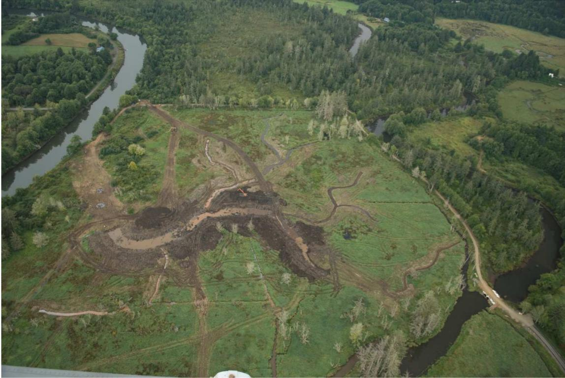
Figure 22. Habitat improvement efforts along the Grays River involve breaching flood-control levees and excavating a tidal channel. These efforts convert an isolated surge plain complex into a lower flooded surge plain and form new tidal channels. Photo C. Cannon, 2013, with aerial support from Lighthawk Aviation.
