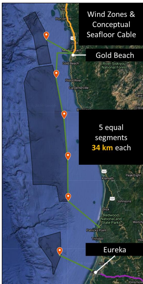
Figure 13: Conceptual AC cable and central wind energy zone configuration
