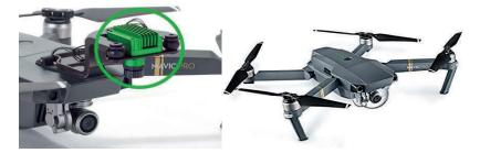
Sentera offers the highly portable DJI Mavic 2 Pro drones, upgraded with High Precision NDVI sensors to produce actionable NDVI data. The Sentera High Precision NDVI Sensors transform the pocket-sized Mavic into an easy-to-use precision scouting tool. The High Precision NDVI sensor enables a grower to capture NIR imagery and produce normalized difference vegetation index (NDVI) crop maps while retaining the ability to use the Mavic's 12-megapixel sensor, capable of shooting 4K video.
