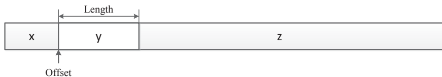
Figure 5.5: The Abstraction of a DMA Record
