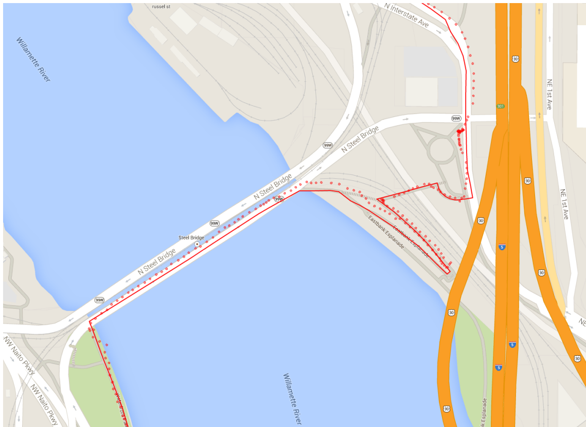
Figure 7: Example of raw GPS coordinates (red circles) compared with matched route (red polyline)
