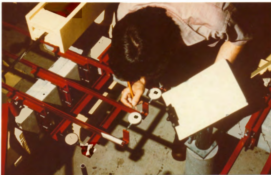
Fig. 4.19. Curvature-meters in position
