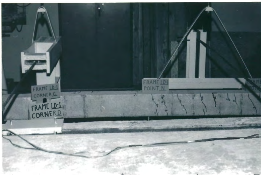
Fig. 5.23. Overall view of frame LD-1 after failure
