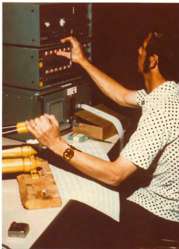
Fig. 4.27. Monitoring loads and pressures with the strain indicator
