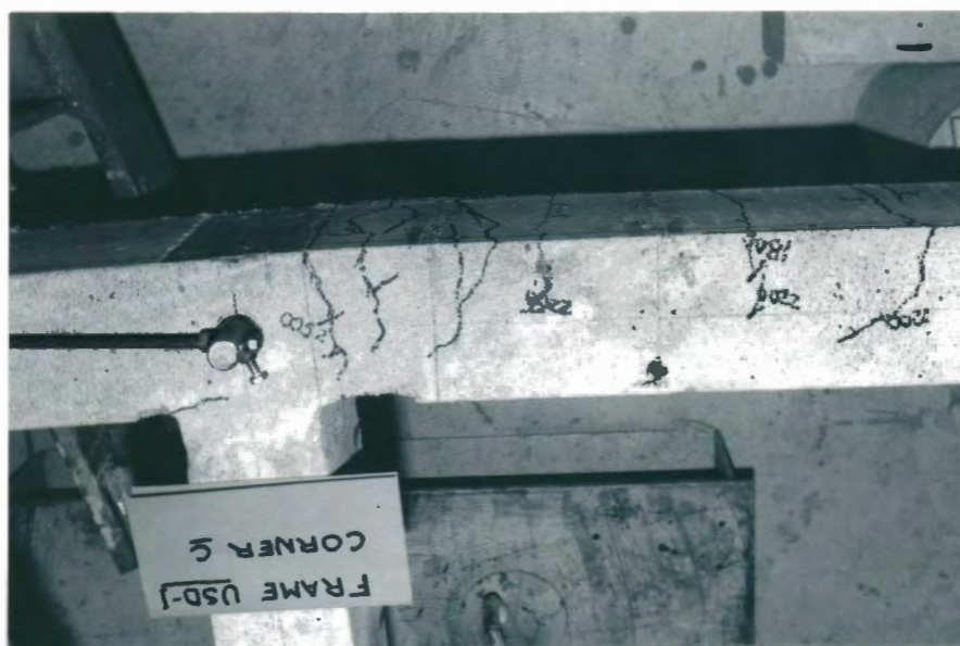
Fig. 5.12. Plastic hinge at corner C
