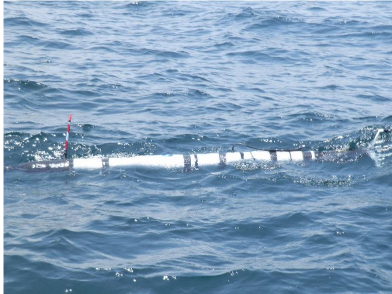
Figure 18. The eFolaga, with the GLASS volumetric array mounted on its nose, beginning one of its missions.
