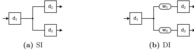
Figure 3.2: Circuit classification depending on the delay model. Square blocks represent gate delay and round blocks represent wire delay.
