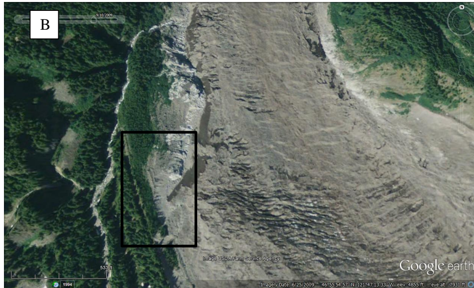
Figure 10. b) Carbon initiation in 2008. The initiation site is a small debris slope and failed into the drainage on the west side of the drainage.
