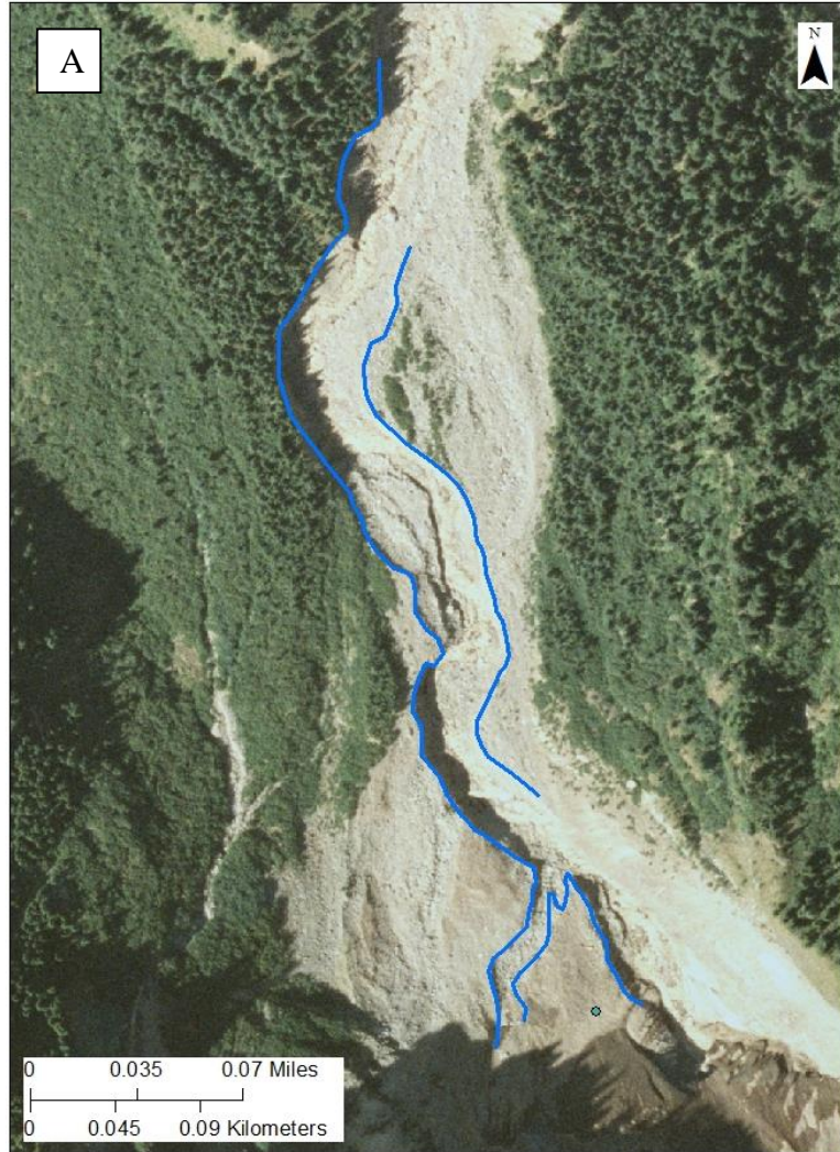
Figure 49. a) 2006 (blue) showing major erosion in the channel margins assumed to be caused by 2006 event which contributed material to debris flow in South Mowich Drainage.
