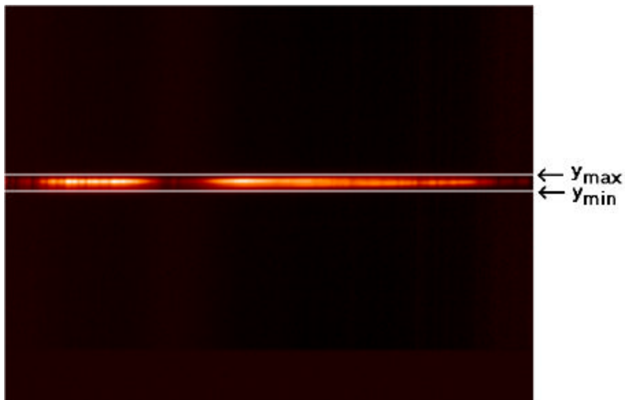
Figure 2-2. The two-sigma threshold estimates for the minimum ( y_{\min} ) and maximum ( y_{\max} ) y-values between which the star spectrum appears.
