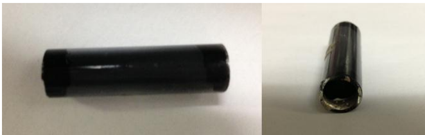
Figure 9: A photograph of fabricated CNT based sensor using method C. Electrical contact to the two sides was provided by using silver epoxy and copper wire as shown in Figure 4.
