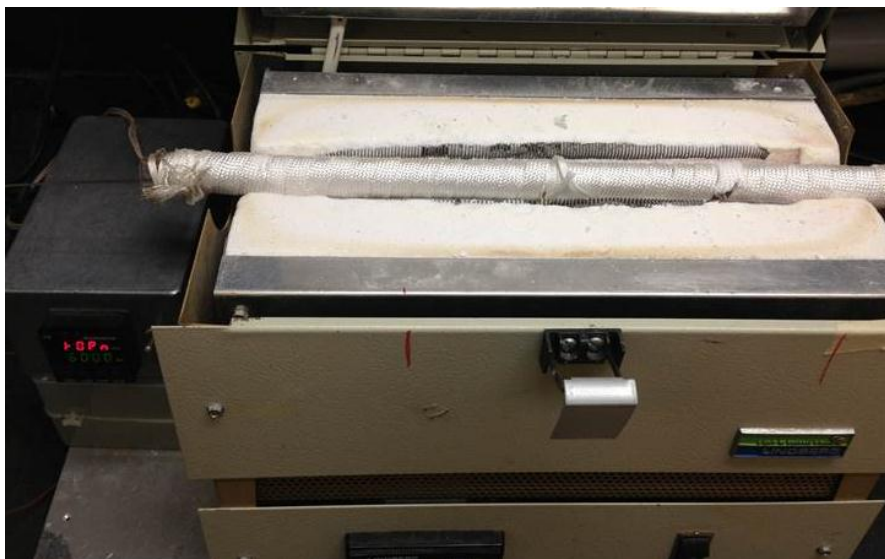
Figure 7: The photograph of the custom-built CNT synthesis system housed inside a tube furnace.
