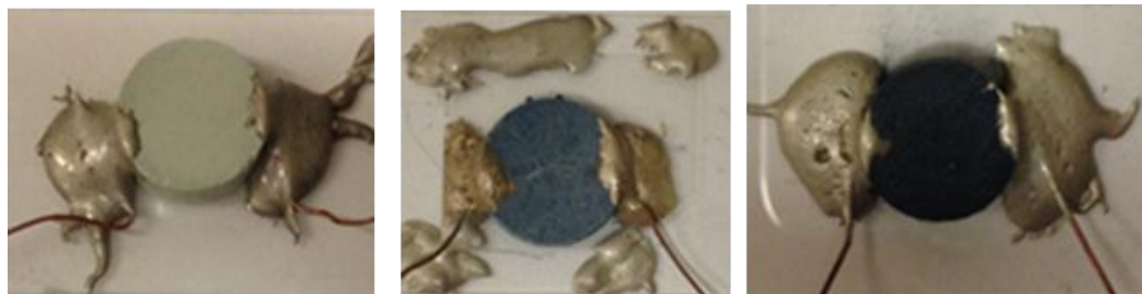
Figure 4: Photographs of 1%, 5% and 10% Sb-doped SnO 2 NWs based sensors (from left to right). Note the increase in the dopant concentration leads to increasingly blueish color to the pellets. Electrical contacts (silver epoxy and copper wire) and compressed nanoparticle pellet are mounted on a microscope glass slide.
