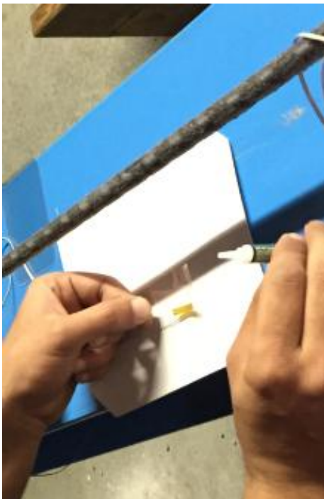
(C) Applying the glue
