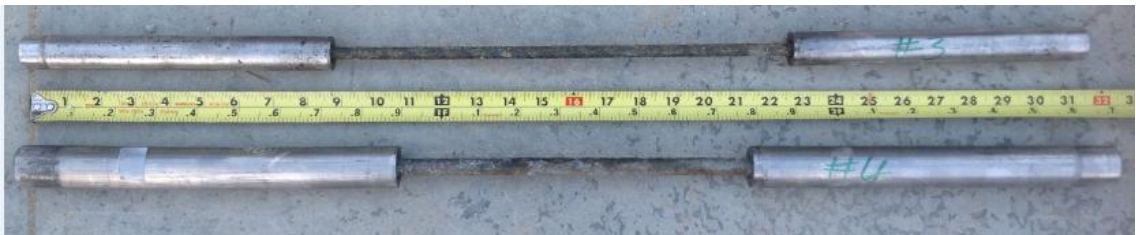
Figure 3.1 Anchored CFRP samples for tensile tests
