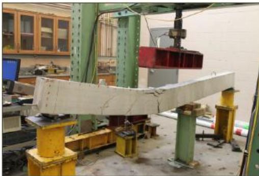
a) CFRP rupture
