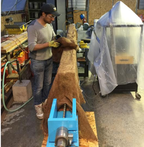
(I) Covering the concrete with wet burlap
