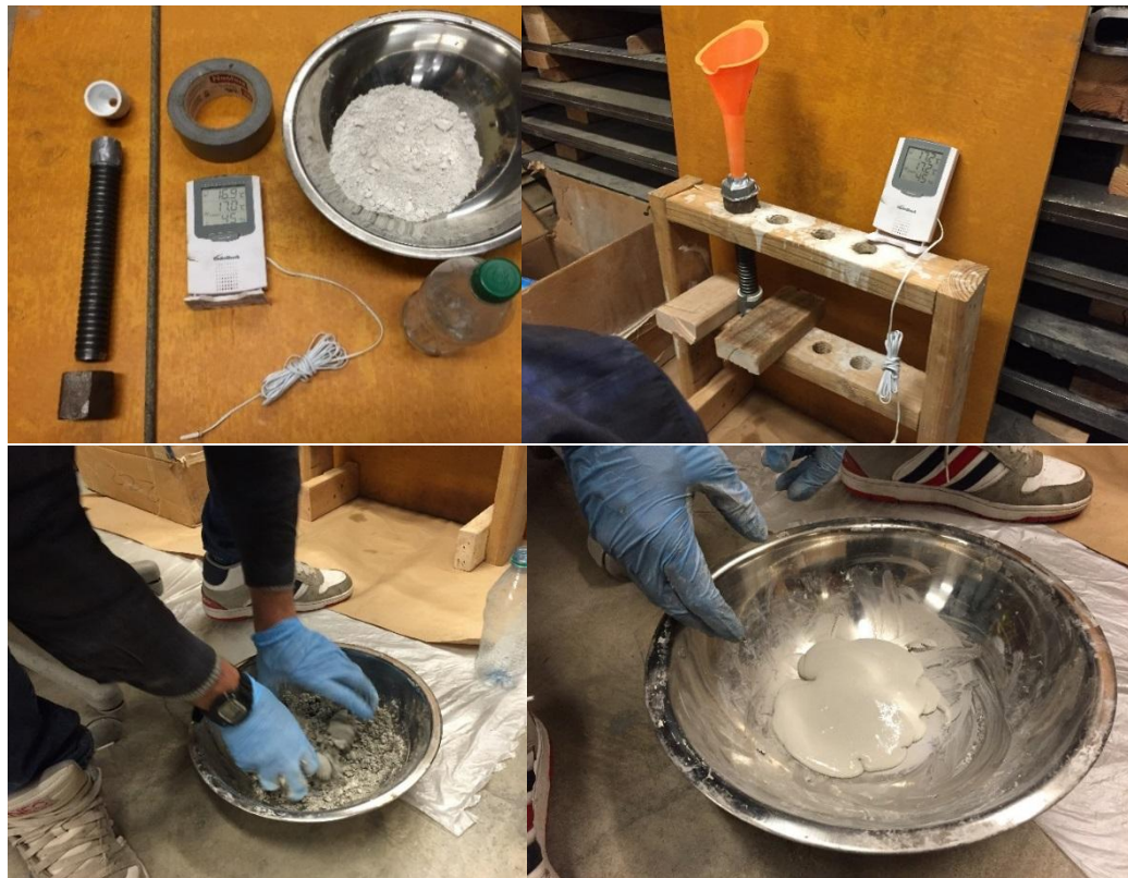
Figure 3.6 Casting process to attach the anchorage steel tube
