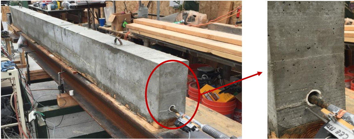
Figure 4.7 Typical view for Beams #1 to #3 showing the un-bonded technique for CFRP at the ends.
