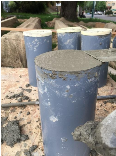
(G) Casting Cylinders
