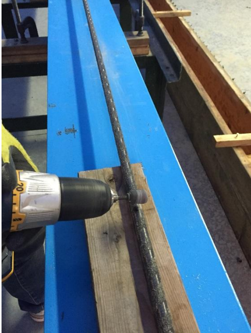
(A) Grinding: creating smooth area on the surface of CFRP strand
