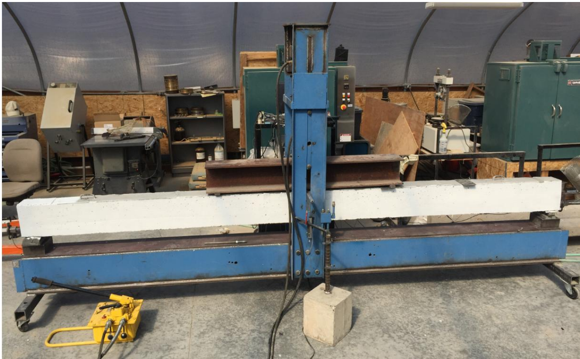
Figure 3.27 Set-up for flexural tests
