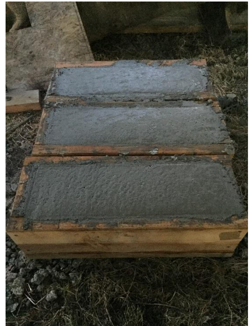
(H) Plain concrete beam for flexural strength test
