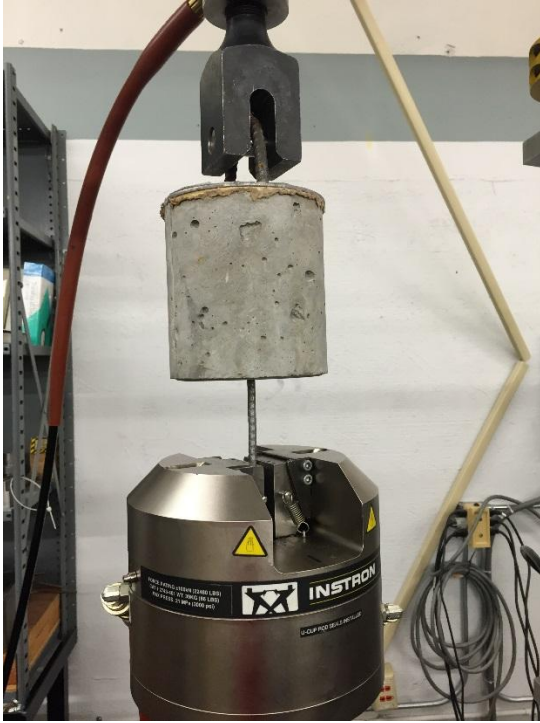
Figure 4.35 D5 vs. concrete bond test
