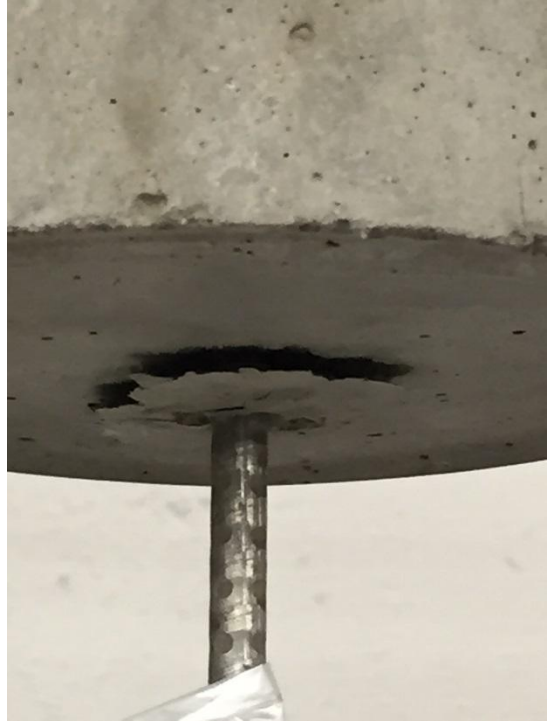
Figure 4.35 D5 vs. concrete bond test
