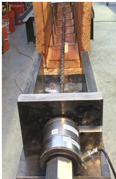
Figure 3.23 Locking the CFRP strand with the load cell at the dead end
