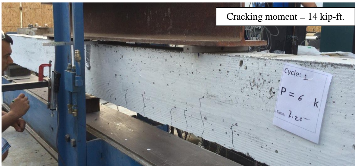
Figure 4.20 Photos of the flexural test of Beam #3
