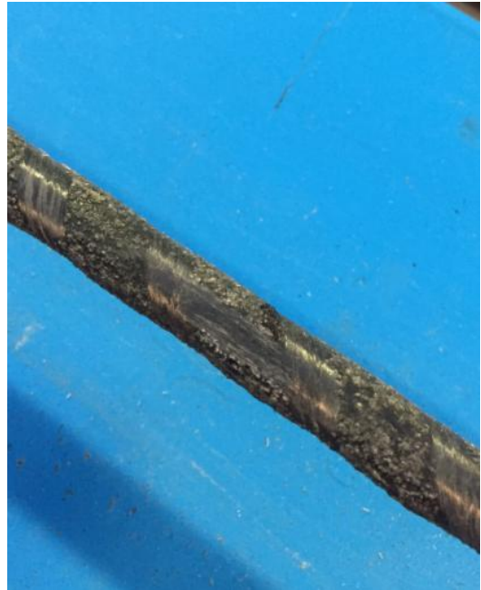
(B) Clean surface for strain gauge to be installed
