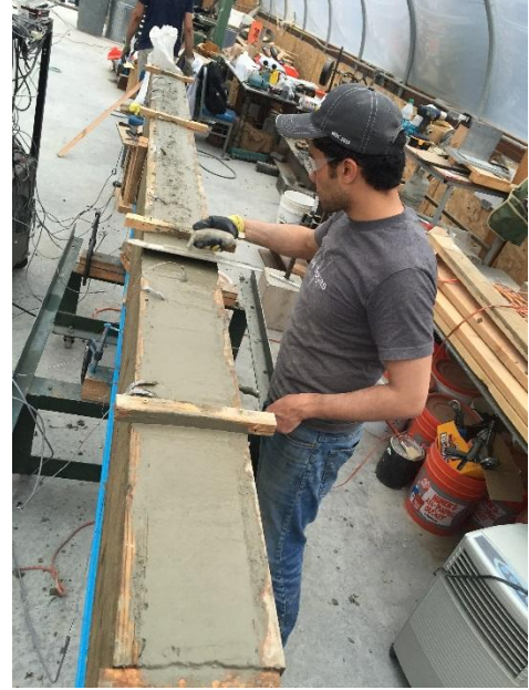
(F) Surface finishing using a trowel
