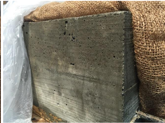
(E) Concrete condition after 12 hours of covering – still wet
