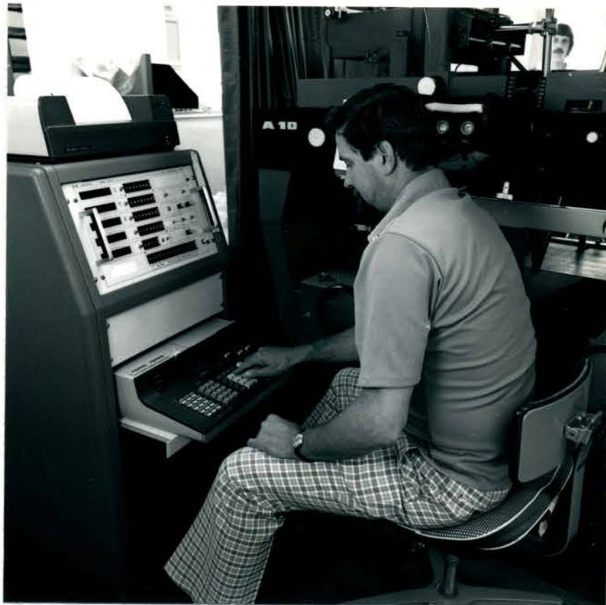
Figure 7. Programmable calculator being operated by photogrammetric technician. Thermal printer on top of digitizing console is interfaced to the calculator to provide a hard copy of calculator output
