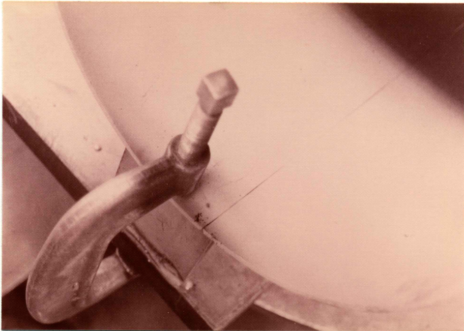
Figure 3.2 Ready for inside weld pass
