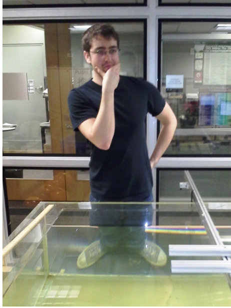
Figure 1.3: Example of refractive distortion. The subject's feet appear significantly displaced from their actual location due to the oblique viewing angle from the surfaces of the water tank.
